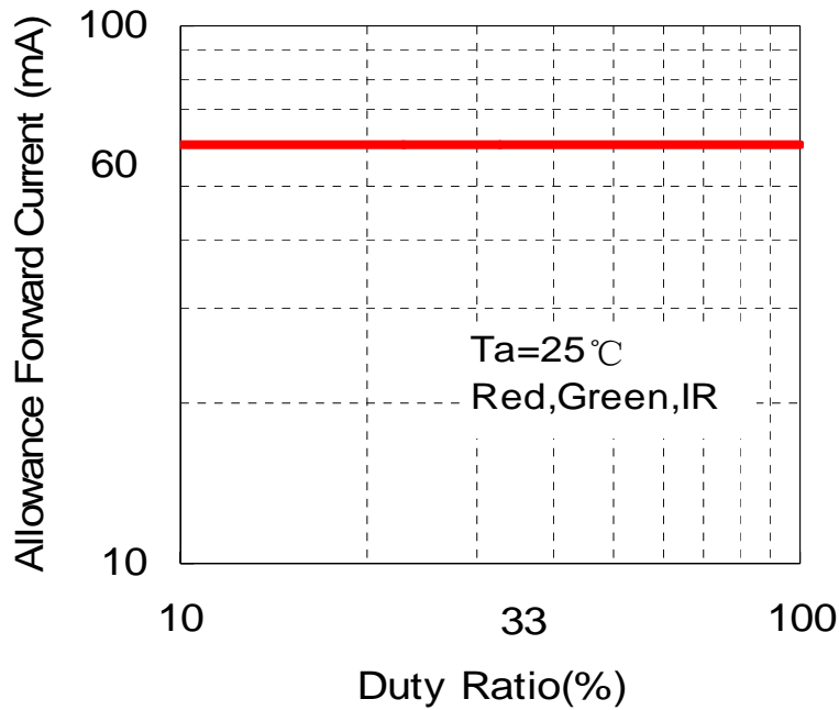
Figure 3. Duty Ratio vs Allowable Forward Current
